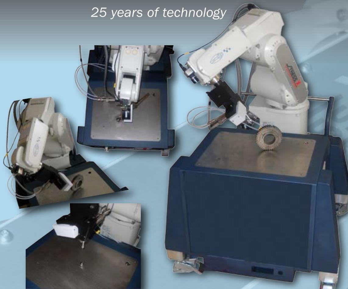
Stress-X allows to measure residual stress, providing a through non-destructive analysis of samples of any dimensions tank to the original mounting of the diffractometer head on a 6 anthropomorphic axis robot.
