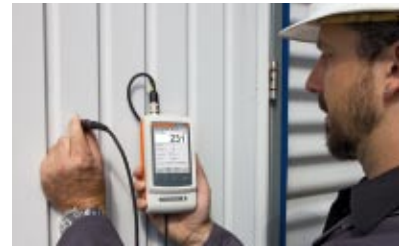
Measurement of paint coating thickness
