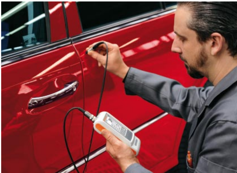
Measurement of auto body paint thickness using the Dual Probe FD10
