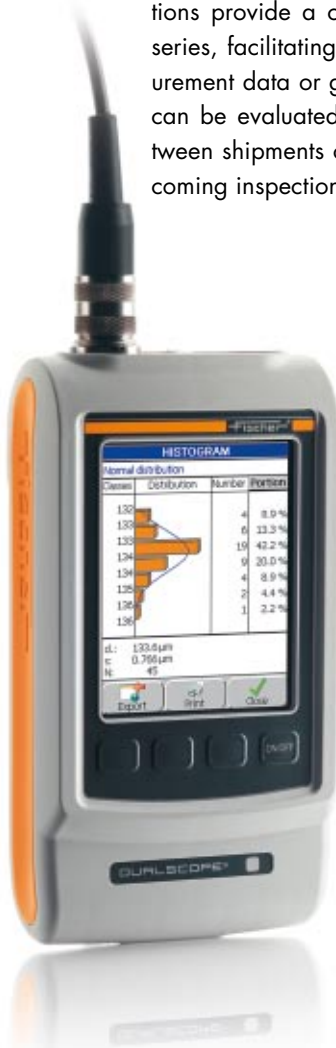
Typical examples of evaluation options, as viewed on the high-resolution LCD colour displays of the DUALSCOPE FMP100 and FMP150 instruments
