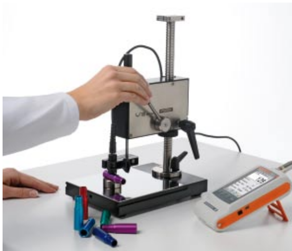
Precise measurement on curved anodised parts using the V12 BASE support stand and the curvature-compensated probe FTD3.3
