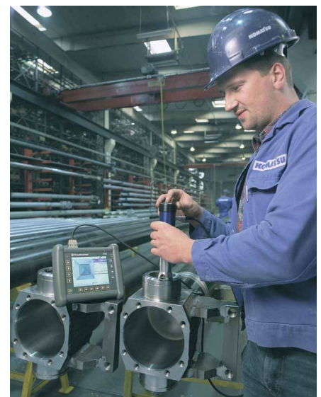
Fig.12: The TIV hardness tester in field use.
