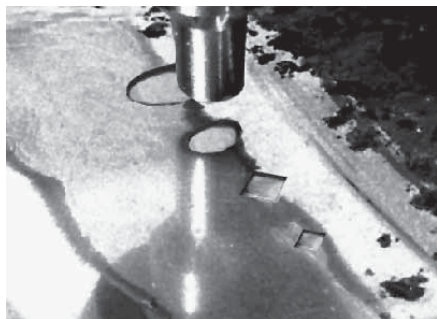
Fig. 24: Hardness testing in the heat-affected zone (HAZ).
