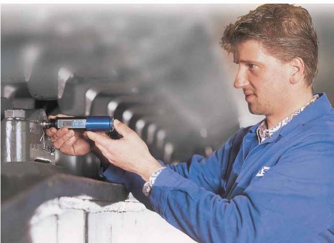
Fig. 3: Hardness testing using the DynaPOCKET on the chain of an open-pit mining excavator.
