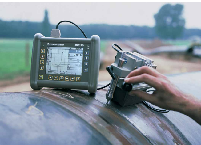
Fig. 1: Hardness testing using the MIC 20 in combination with the test support MIC 227 and a UCI probe in the heat-affected zone (HAZ) of a weld.
