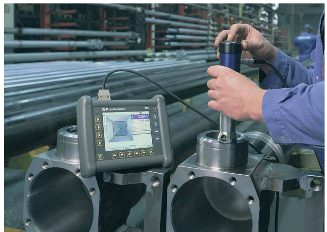
Fig. 4: Optical hardness testing using the TIV tester. Checking before final assembly.
